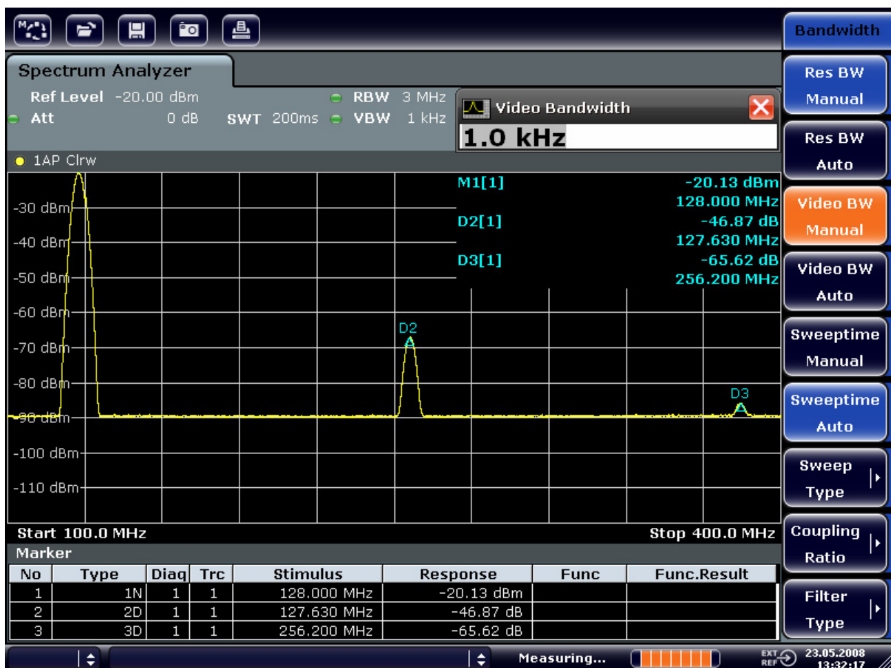
Figure 10: Suppression of noise during harmonics measurement by reducing video bandwidth
